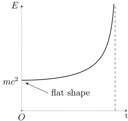
Figure 4:  $E$  vs  $v$  for a massive particle
