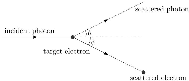
Figure 5: The schematics of Compton scattering
