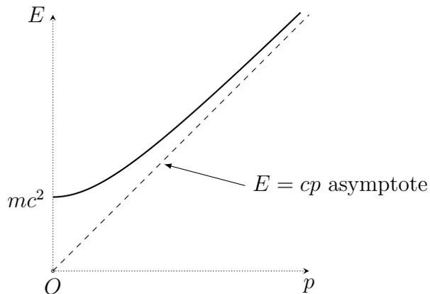
Figure 1:  $E$  vs  $p$  for a massive particle
